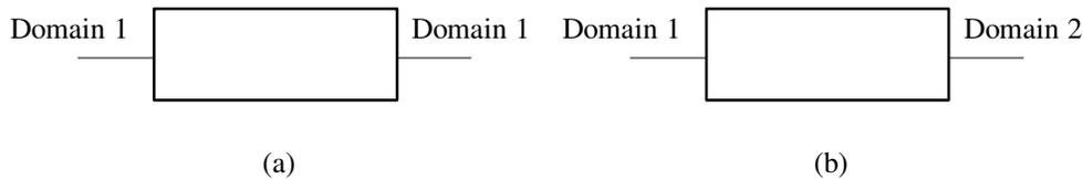
Fig. 4-1 A modifier (a) and a transducer (b)
