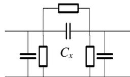
Fig. 5-4 Reduced electrical model at low frequencies
