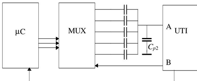
Fig. 6-18 Block diagram of the system using the UTI from Smartec
