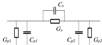
Fig. 5-13 Electrical model in the case of slightly conducting fluids in direct contact with the electrodes
