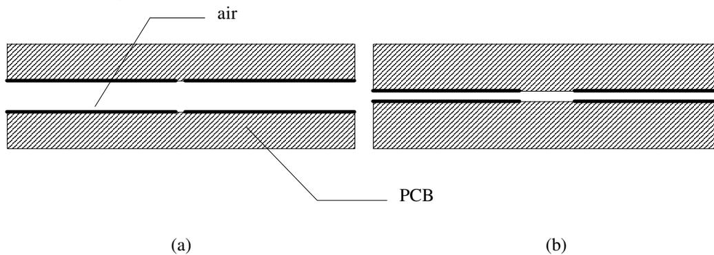
Fig. 5-18 Cross-capacitors with thin electrodes on printed circuit board, (a) with thin gaps and (b) with wide gaps
