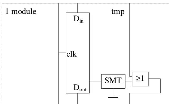
Fig. 8-8 Multiplexer circuits for Smartec temperature sensors
