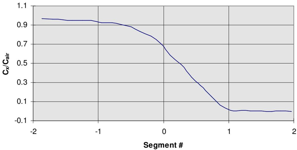
Fig. 8-9 Measured capacitance ratio versus interface level for conductive liquids
