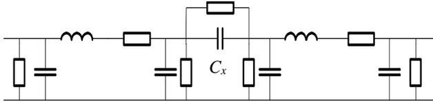
Fig. 5-3 An example of the electrical model of a multi-electrode structure at higher frequencies using the quasi-static approximation
