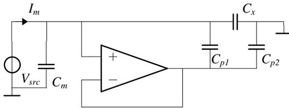
Fig. 6-3 1-port measurement with active guard
