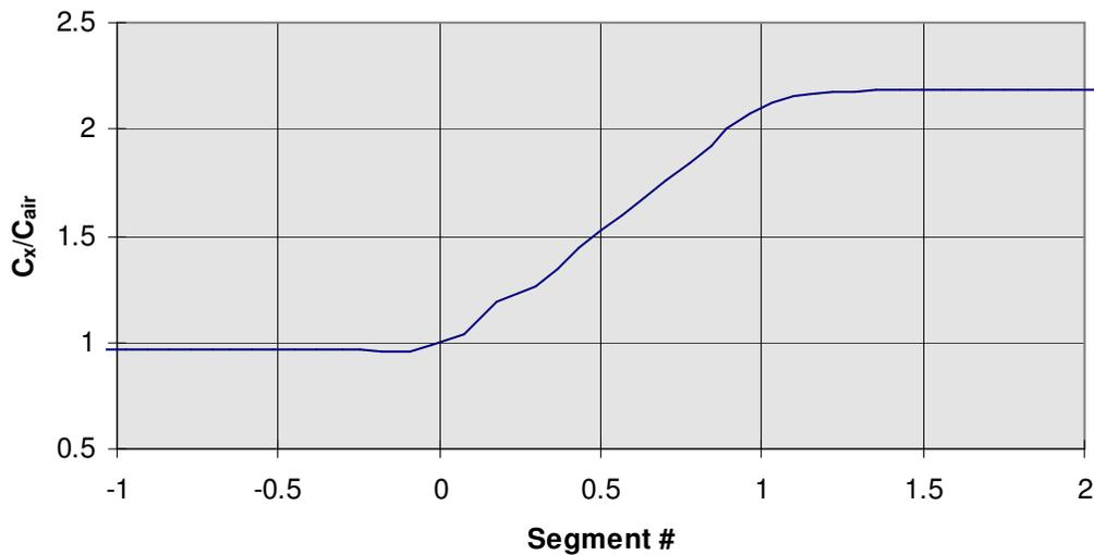
Fig. 8-10 Measured capacitance ratio versus interface level for non-conductive liquids
