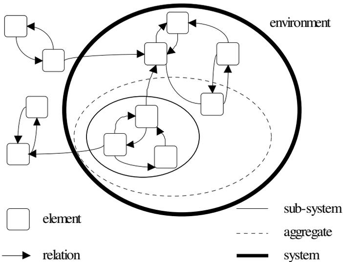
Fig. 3-1 System, aggregate and sub-system
