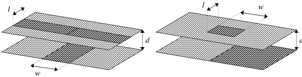
Fig. 5-9 Differential biplanar electrode structures
