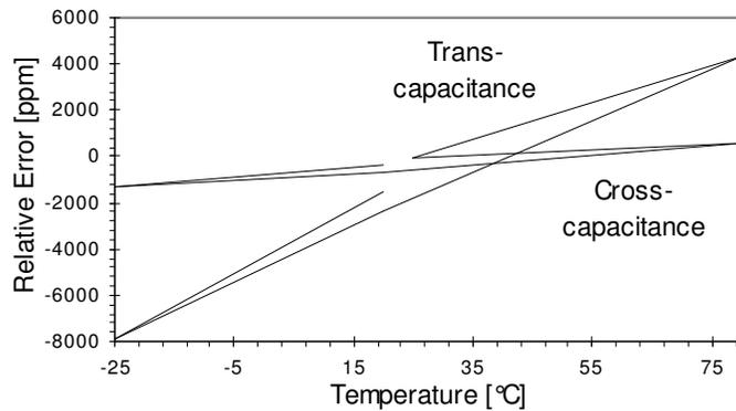
Fig. 7-29 Temperature effects on the circular cross-capacitor and the circular trans-capacitor
