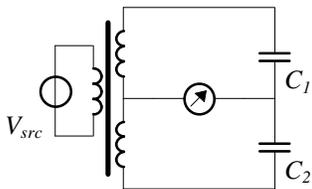
Fig. 6-7 Bridge circuit with 3-winding transformer
