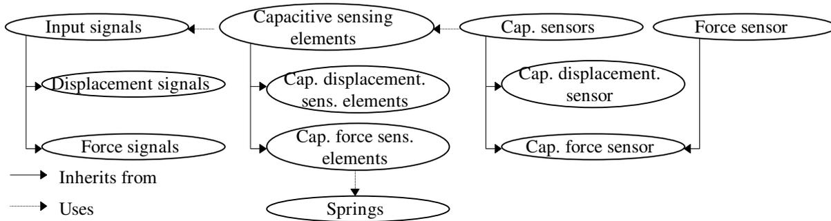
Fig. 7-21 Class diagram for capacitive displacement and force sensors and sensing elements
