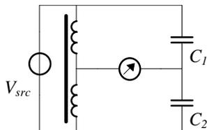
Fig. 6-6 Bridge circuit with 2-winding transformer
