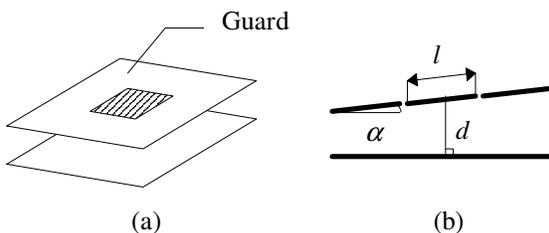
Fig. 5-8 Parallel plate capacitor (a) perspective (b) cross-section
