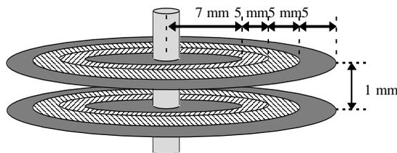
Fig. 5-21 Experimental circular cross-capacitor
