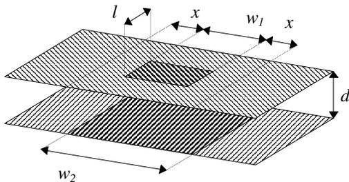
Fig. 5-15 Biplanar square-strip geometry
