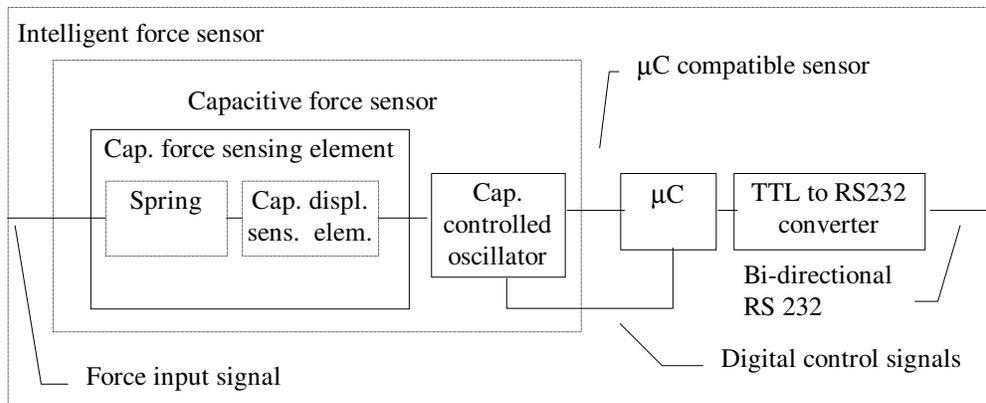
Fig. 7-23 Data flow diagram for an intelligent force sensor
