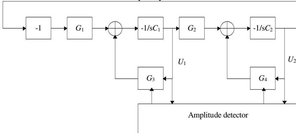
Fig. 6-12 Two-integrator oscillator
