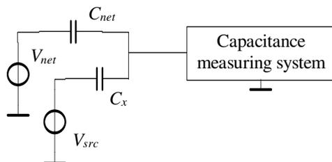
Fig. 6-5 Electrical model for LF interference
