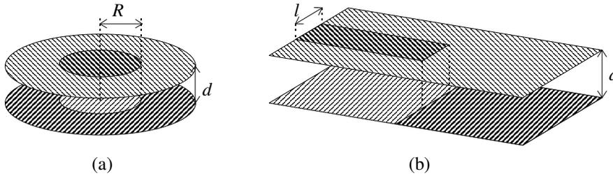
Fig. 5-7 (a) Circular and (b) linear biplanar cross-capacitor
