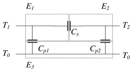
Fig. 5-2 Static electrical model for a multi-electrode capacitor
