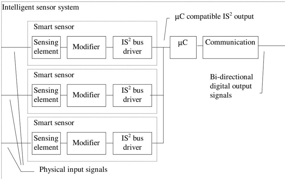
Fig. 4-8 Generic data flow diagram for an intelligent sensor system with IS<sup>2</sup> bus
