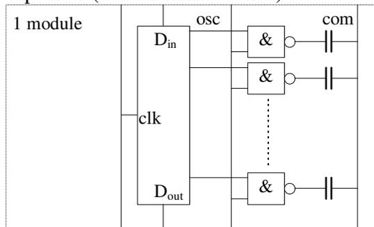
Fig. 8-7 Multiplexer circuit for capacitances
