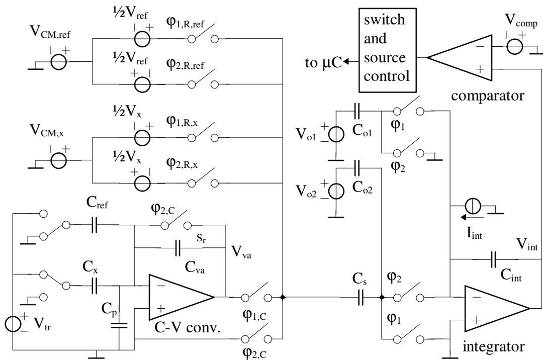
Fig. 6-17 Multiple-sensor modulator in capacitance measurement mode (reprinted from [79])
