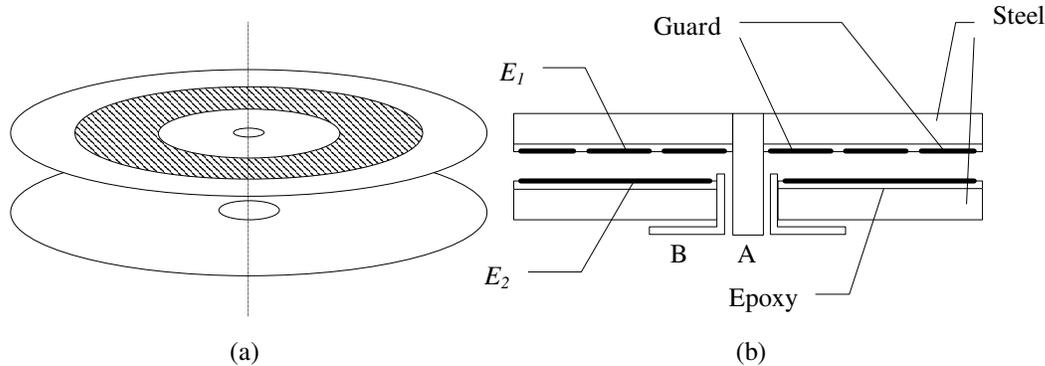
Fig. 7-24 The proposed capacitive sensing element (a) perspective (b) cross section
