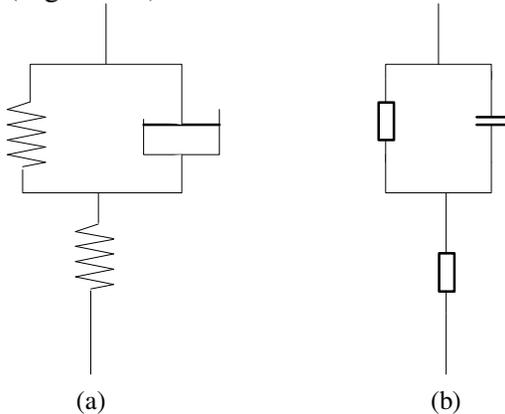
Fig. 7-26 Mechanical (a) and equivalent electrical model (b) for time-dependent anelastic deformation
