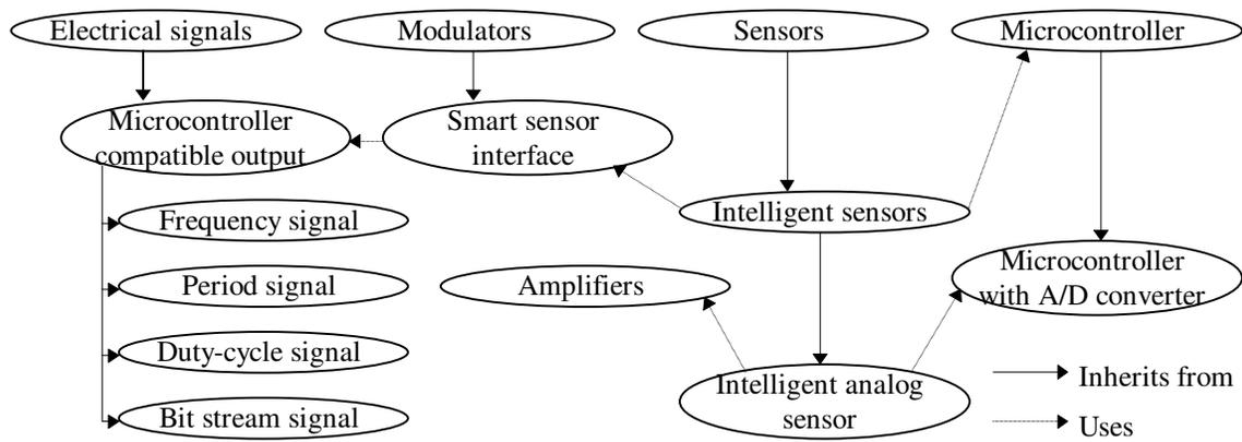
Fig. 4-5 Class diagram for intelligent sensors
