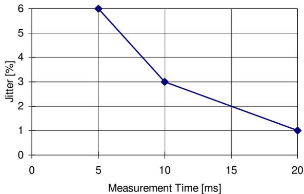
Fig. 9-8 Jitter of the measurement system versus measurement time
