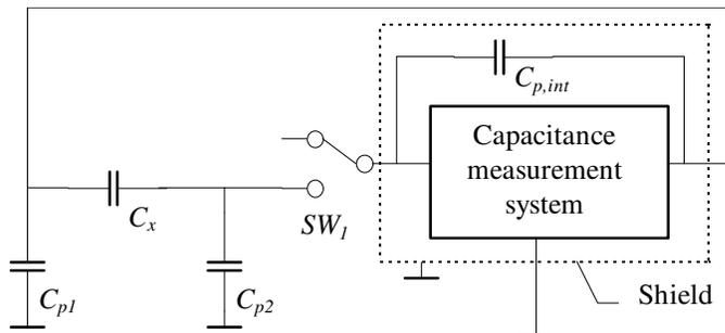
Fig. 6-1 Identification of parasitic capacitances
