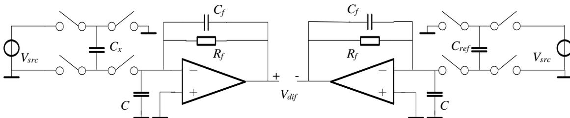
Fig. 6-10 Charge/discharge method
