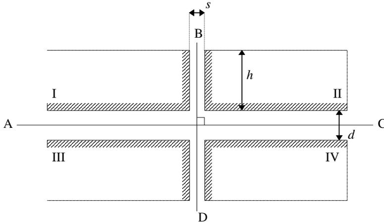
Fig. 5-16 Cross-section of a cross-capacitor with infinite deep gaps
