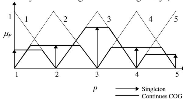
Fig. 9-7 Defuzzification using singletons
