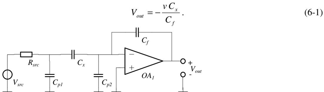
Fig. 6-2 Circuit to reduce the influence of  $C_{p2}$  and  $C_{p3}$
