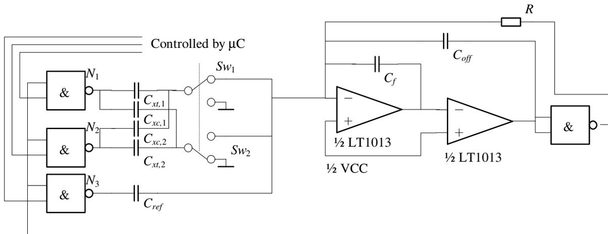
Fig. 6-15 Martin oscillator with double-sided multiplexing
