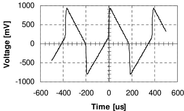
Fig. 6-14 Measured output signal of the integrator
