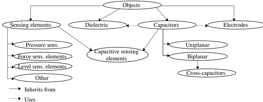
Fig. 5-24 Class diagram for capacitive sensing elements
