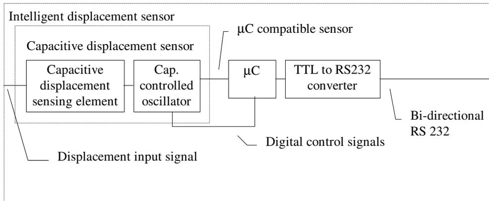
Fig. 7-22 Data flow diagram for an intelligent displacement sensor
