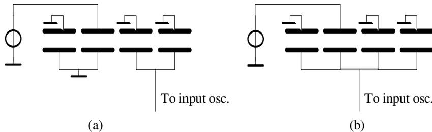
Fig. 5-22 Right-half cross-section of the electrode structure for measuring (a) cross-capacitance and (b) trans-capacitance
