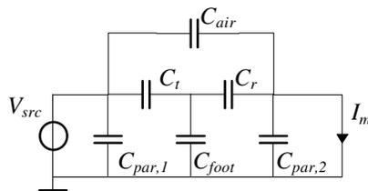
Fig. 9-2 Simple electric model of the structure
