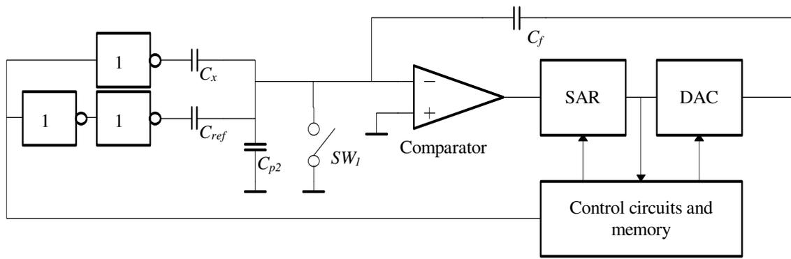
Fig. 6-11 Charge amplifier presented by Kung *et. al.*
