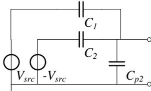
Fig. 6-8 Bridge imbalance measured with a voltage meter
