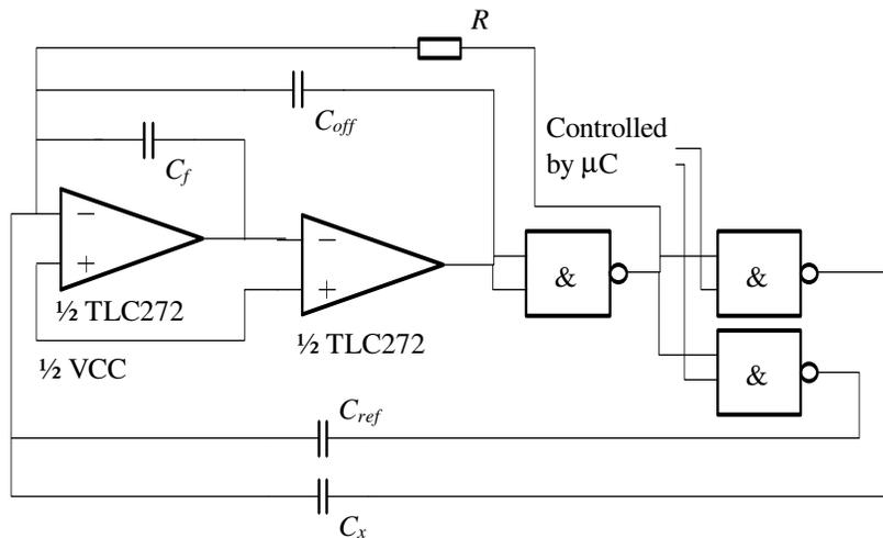
Fig. 8-6 The modified Martin oscillator
