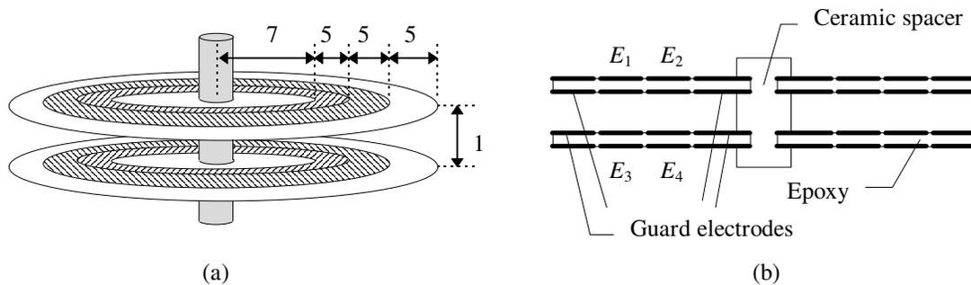
Fig. 7-25 Proposed circular cross-capacitor (a) perspective (b) cross-section
