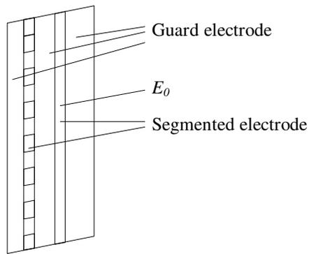
Fig. 8-5 Novel planar electrode structure
