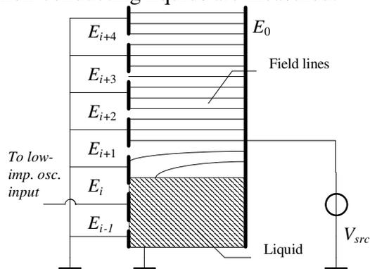
Fig. 8-4 Conductive liquid connected to ground
