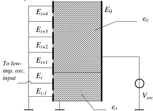
Fig. 8-3 Multi-electrode structure where  $C_i$  is measured
